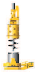
Cased Kelly drilling (installation with oscillator)
