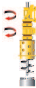
Cased Kelly drilling (installation with BTM)
